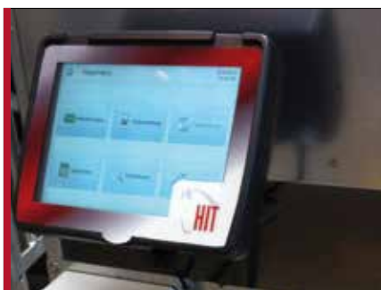
HOCO-Foderstation styr hela fodersystemet
