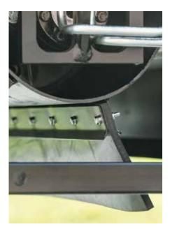
With its 6 lips made from fabric-reinforced, high-performance rubber, the sweeping roller has a hydraulic drive.
